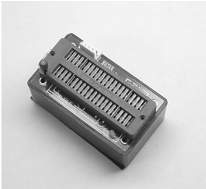
Figure 3.17 USB PIC programmer by Micropro.
