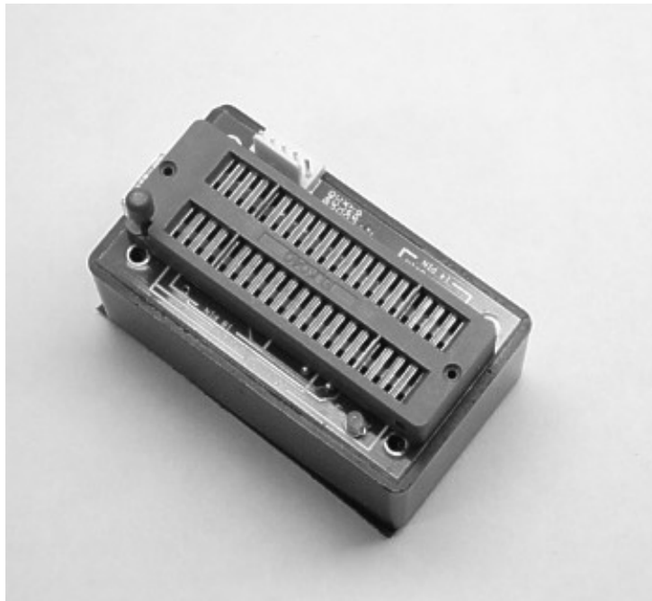
Figure 1.1 USB PIC programmer made by MicroPro.
